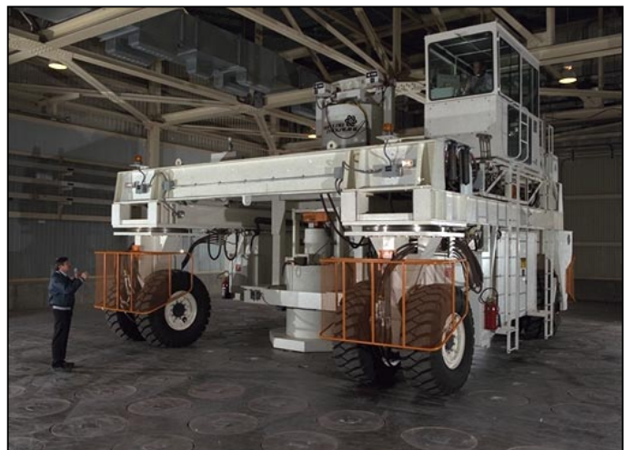
The Shielded Canister Transporter (SCT) moves highly radioactive canisters from DWPF to the GWSB. The SCT removes a round shield plug from the floor, lowers the canister into a vertical storage position, and replaces the shield plug.
