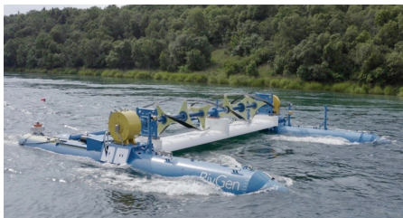
The ORPC RivGen Power System prior to installation on the Kvichak River in Igiugig, Alaska. Source: ORPC
