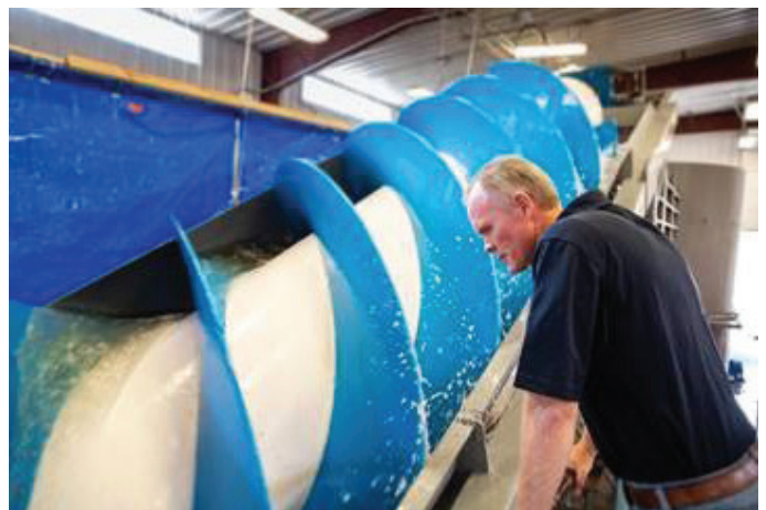
Percheron Power's composite Archimedes hydrodynamic screw. Source: Utah State University
