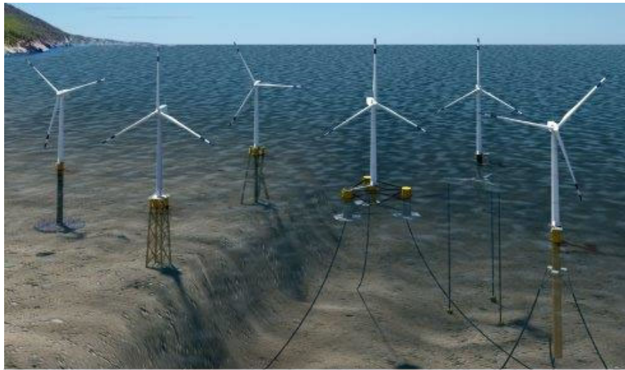
U.S. offshore wind projects are developing a variety of different foundations suited to unique conditions at each site. Illustration by Josh Bauer, National Renewable Energy Laboratory (NREL)
