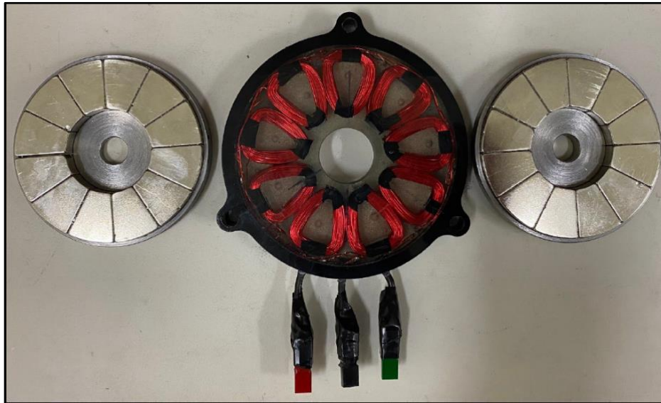
Figure 14. WiscWind's stator and two rotors
