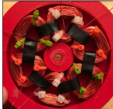
Figure 6: Second & current stator design
