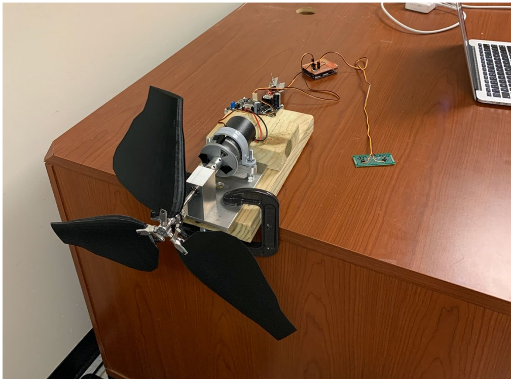
Figure 3: Dynamometer and controls for rotor stress test
