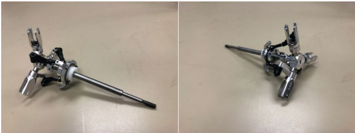
Figure 1: Rotor and pitch mechanism with Delrin filler
