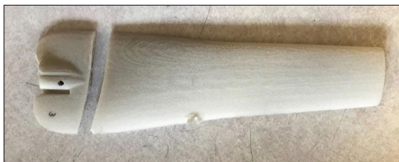
Figure 7 Critical failure at max load
