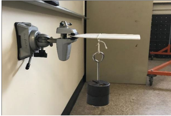
Figure 6 Benchtop Test for Nylon 12 Blade
