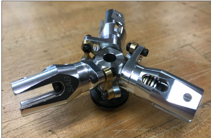
Figure 9 Repurposed rotor hub for turbine blades
