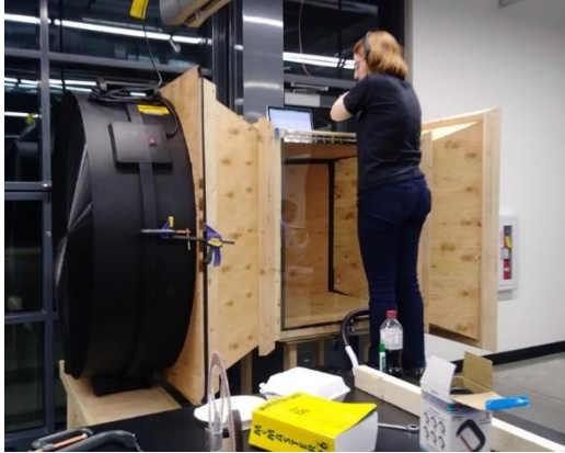
Figure 20: Wind tunnel constructed for runaway test
