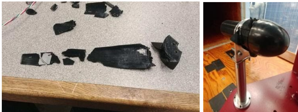
Figure 17: Remaining blades and hub (left) and nose cone (right) after rotor strength test in wind tunnel.
