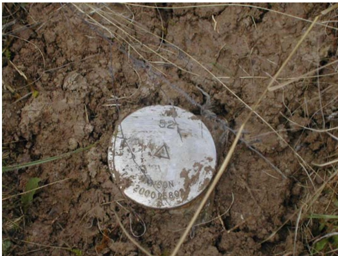
Photo 5. Groundwater restriction boundary monument WS-52. Dirt was replaced around monument.
