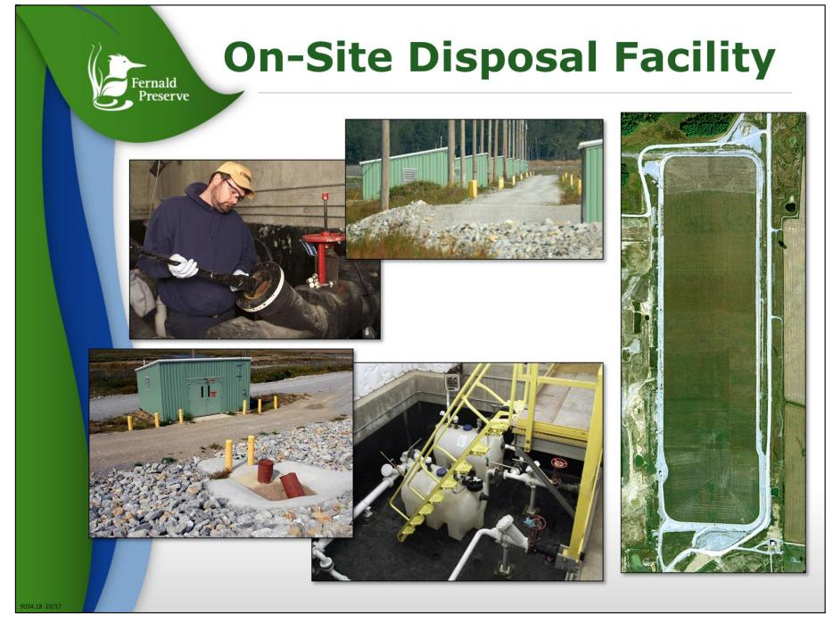
The On-Site Disposal Facility is an engineered waste-storage area that holds 2.95 million cubic yards of waste that was generated as part of the site cleanup.
