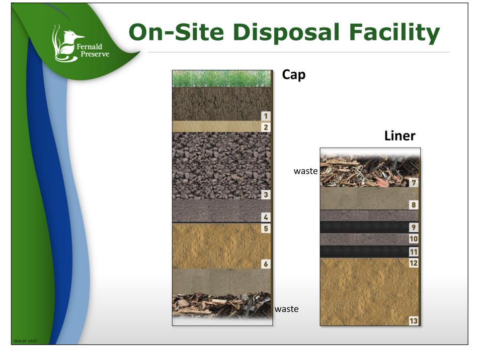
Waste is safely encapsulated between a 9-foot cap and a 6-foot liner within the On-Site Disposal Facility.
