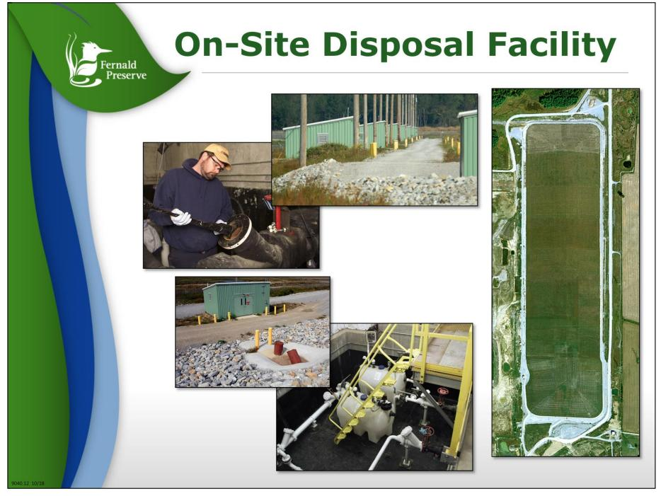
The On-Site Disposal Facility (OSDF) is an engineered waste storage area that holds 2.95 million cubic yards of waste (85 percent soil and soil-like material, and 15 percent demolition debris) that was generated as part of the site cleanup.
