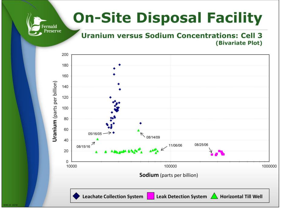
A comparison of uranium concentrations and sodium concentrations in and below Cell 3 of the OSDF is an example of a method used to demonstrate the liner system is working as designed.
