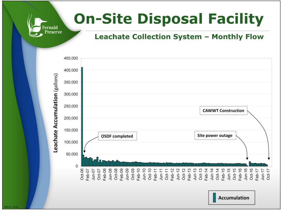
Leachate is the moisture in the waste within the OSDF and includes water sprayed on the waste to control dust and rainfall events prior to cell capping. The leachate is collected and transferred to an on-site treatment facility. Before the cover system was completed in October 2006, hundreds of thousands of gallons of leachate flowed each month.
