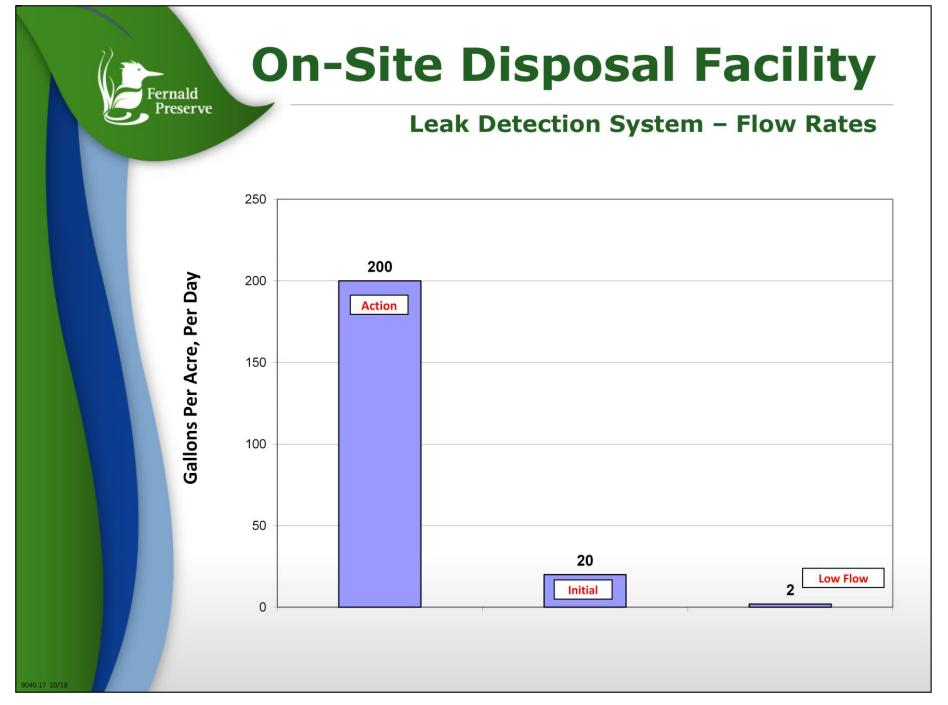
By design, monitoring flow from the Leak Detection System is one of the main indicators of whether or not the facility is operating as designed.
