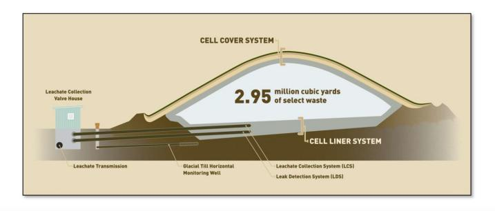
The OSDF was constructed with an engineered liner and cover system that serves to isolate the entombed waste from the environment.
