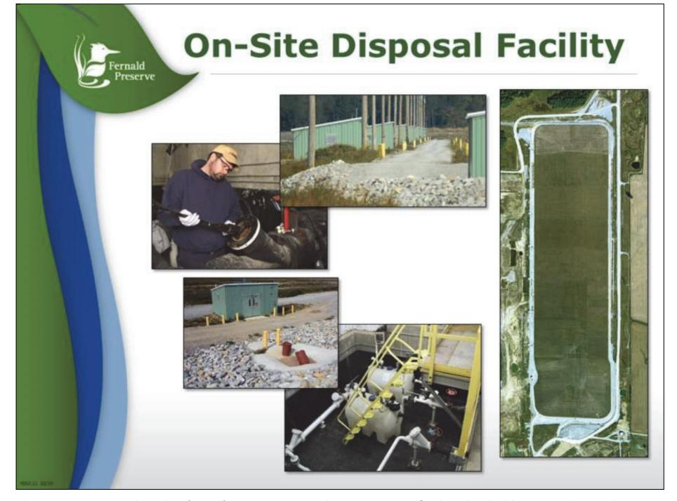
The On-Site Disposal Facility (OSDF) is an engineered waste storage facility that holds 2.95 million cubic yards of waste (85% soil/soil-like material and 15% demolition debris) that was generated as part of the site cleanup.
