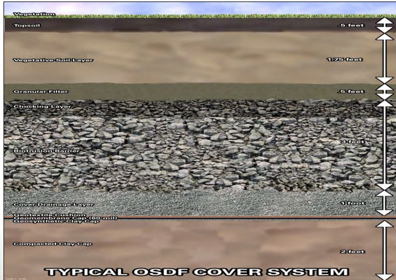
The OSDF engineered cover system.
