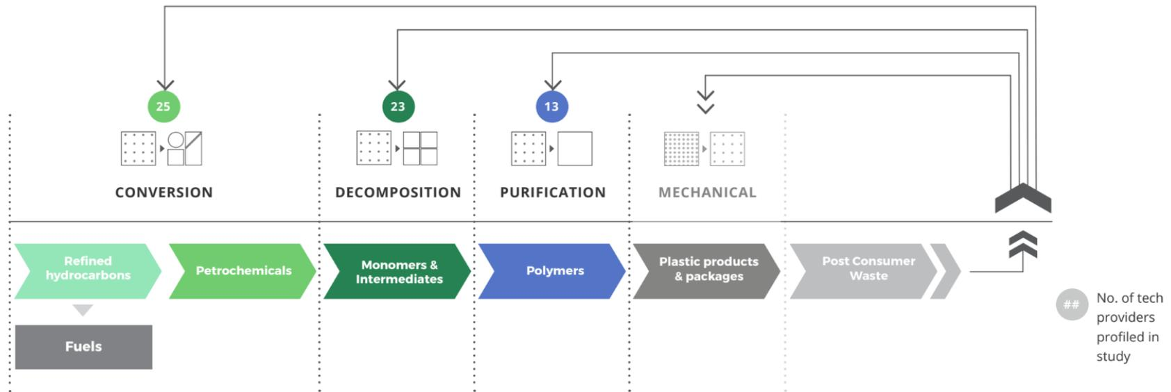
**Conversion:** a thermal process involving breaking bonds in the polymer to produce liquid and gaseous products such as fuels and petrochemicals.
