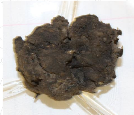
(a) Raw dry MSW digestate
