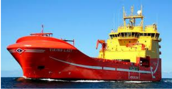
Viking Lady 330kW fuel cell – 18'500rhs 500kWh ESS
