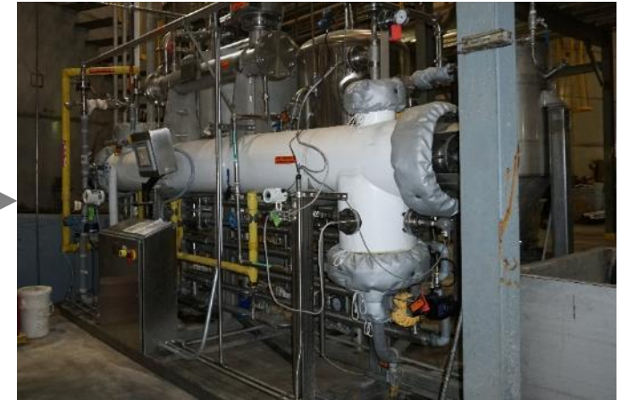
Pretreatment Reactor: Acid + heat + time
