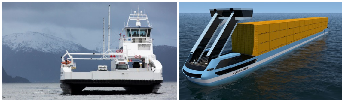
Figure 10.2. The first all-electric ferry operating in Norway, the MF Ampere (left) and the Port-Liner fully electric canal cargo vessel in development and capable of autonomous operation (right). Sources: www.siemens.com/press and Port-Liner
