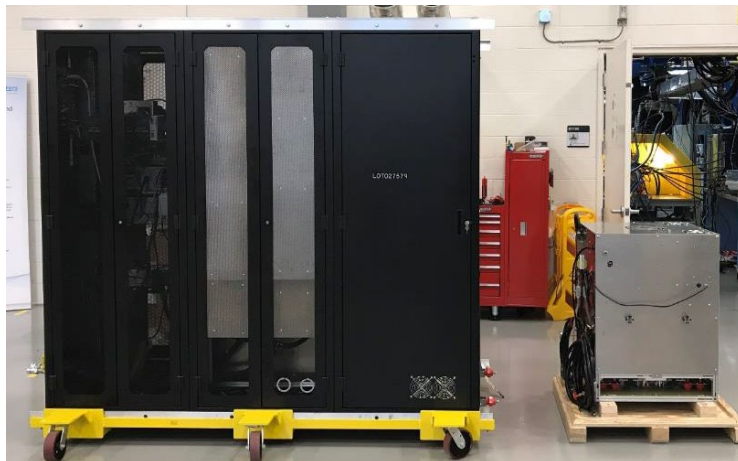
Si IGBT inverter ~5,500 lbs, ~95% eff.
