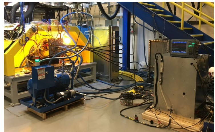
Dynamometer test stand with PM machine and SiC inverter
