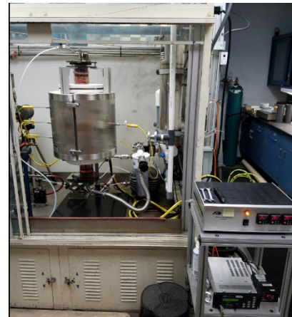
CVI reactor setup at ORNL
