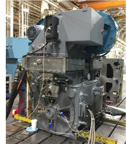
1 MW 15,000 RPM TECO Motor
