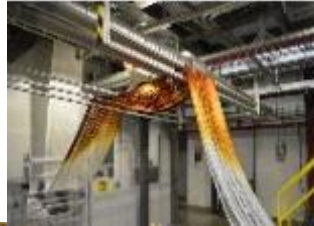
Splicing Method for heavy tows Team: ORNL
