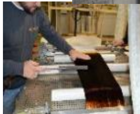
Splicing Method for heavy tows Team: ORNL
