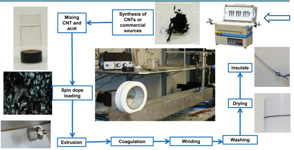
Our approach: scalable & allows independent optimization of CNT synhesis & fiber spinning UNIT OPERATION approach: each step can be optimized separately Cost aspect:
