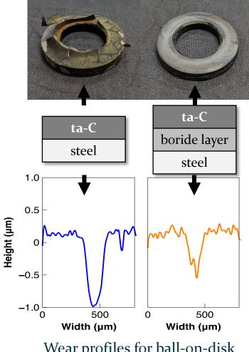
Wear profiles for ball-on-disk experiments (ta-C vs. ta-C)
