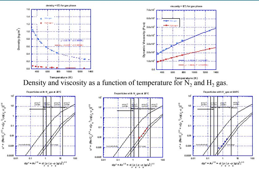
Fluidization map for iron powder. In b) experimental results from are placed on the map with N<sub>2</sub> gas at 20°C and are in excellent agreement (< 10%) with the predicted fluidization behavior. In c) predictions are made for iron powders with H<sub>2</sub> gas at 900°C.<sup>7</sup>
