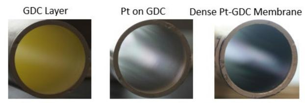
Tubular Nano-Layered Oxygen Separation Membranes
