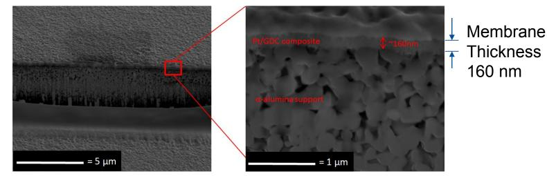
High angle images of deposited membrane layers
