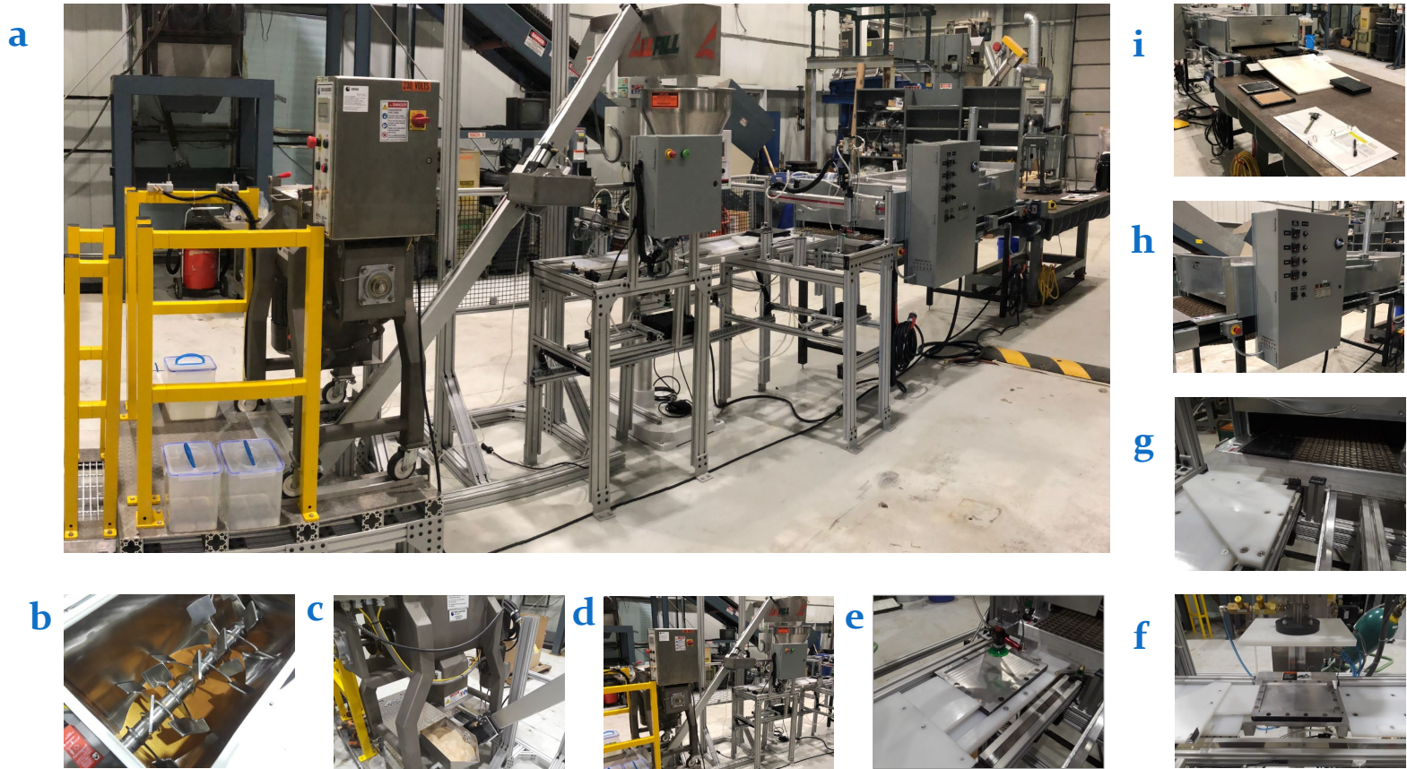
a) semi-automated wafer assembly system including b) mixer, c) bucket, d) pneumatic lift, e) vacuum cups, f) dispenser, g) moving belt, h) infrared oven, i) heat-cured wafers
