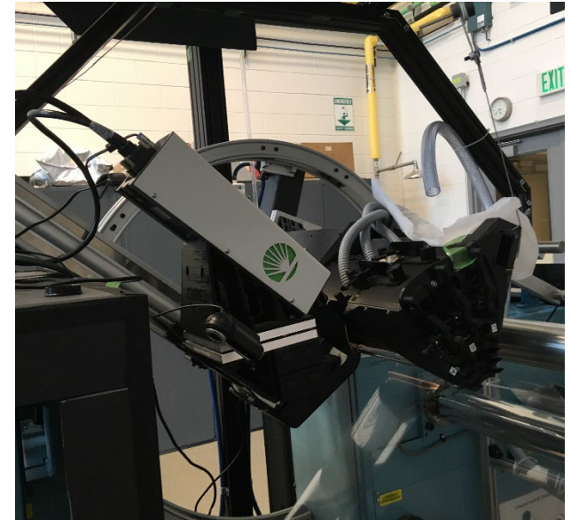
NREL metrology web-line with multi-spectral imager, multiple light source, and membrane web path (below) in a reflectance configuration for thickness imaging
