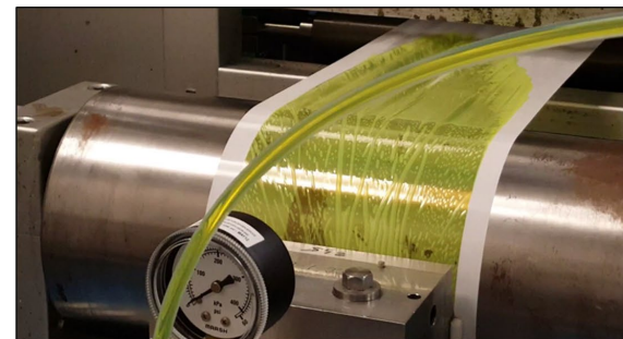
Figure 7. Slot Die Production Coating of PIM-1
