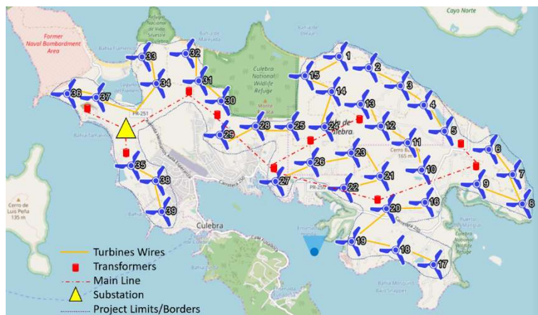
Figure 5: Electrical Plan for the wind farm.
