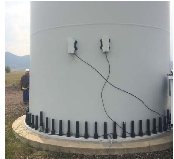
Thermal video cameras installed at the base of a wind turbine (Photo by Bethany Straw)
