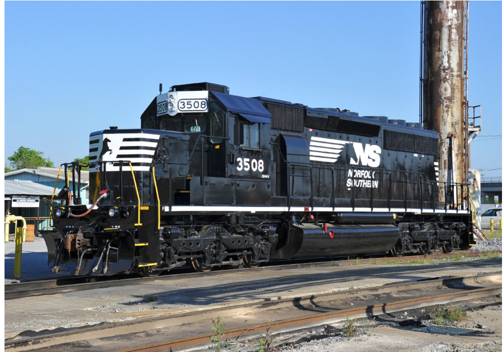
EMD SD40-2 A Typical 6 Axle Yard and Local Locomotive
