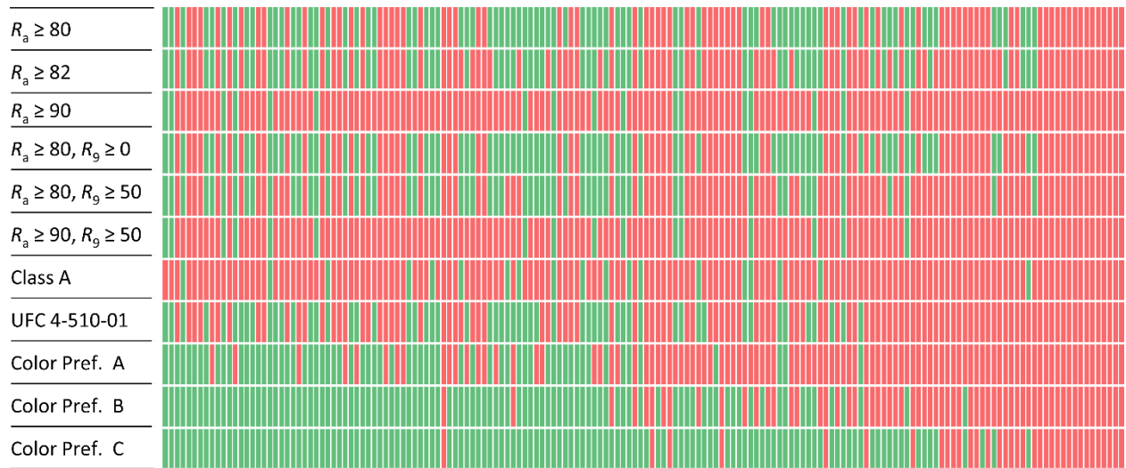
Figure 4. Performance of color rendition specification criteria for the combined Royer et al. dataset [10, 23, 24]. Each bar represents one SPD. The SPDs are arranged in rank order from most preferred (left) to least preferred (right).
