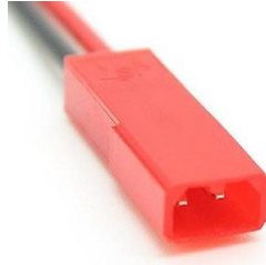
Figure 7. Team-provided connection to the manual shutdown interface
