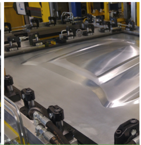
The RAFFT machine built in the first year of the project is on the left. On the right is a 0.4 scale Mustang hood, still in the machine clamp, formed using the RAFFT machine. Photo credit Ford Motor Co.
