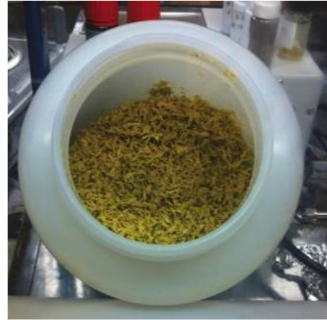
Adhesive polymer binder before being blended with silicon in a slurry process to form improved anode material for Li-ion batteries. [Photo: Berkeley Lab]
