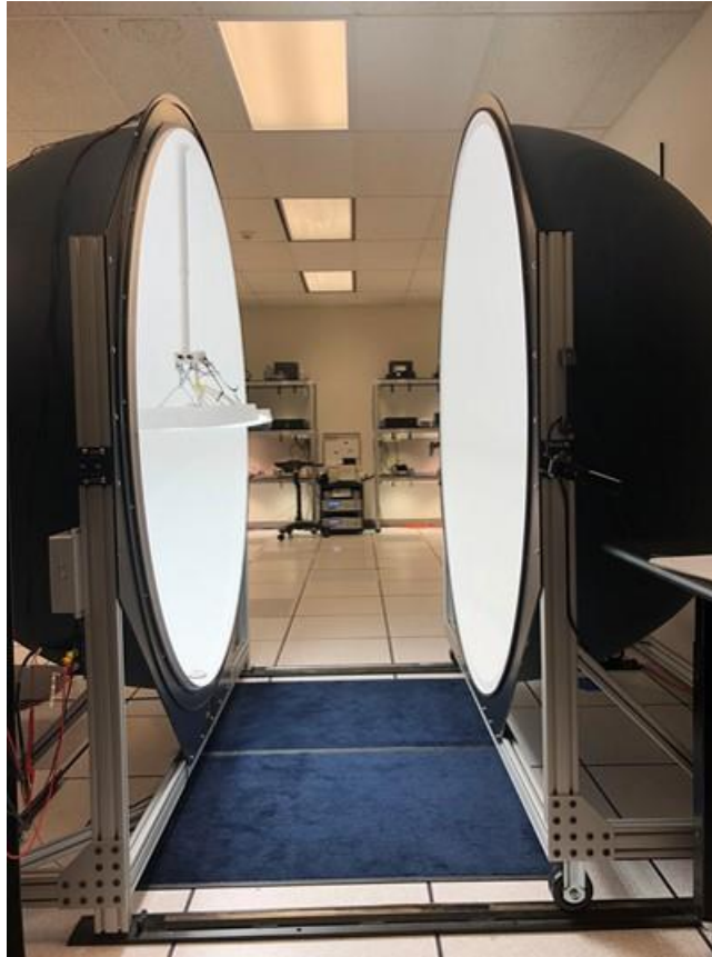
Figure 2. One of the Top Efficacy Performer luminaires in the process of laboratory sphere testing. Photo: PNNL.
