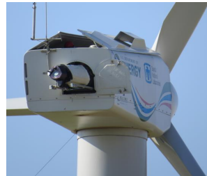
DTU-Wind LIDAR mounted in SWiFT turbine nacelle
