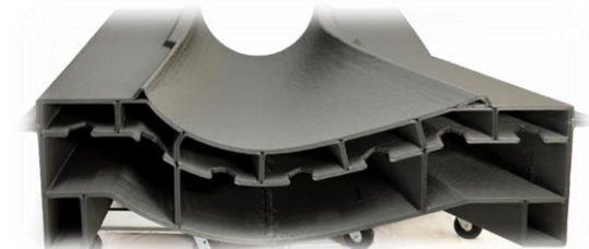
Wind turbine blade mold section manufactured on the BAAM-CI from 20% CF-ABS pellets
