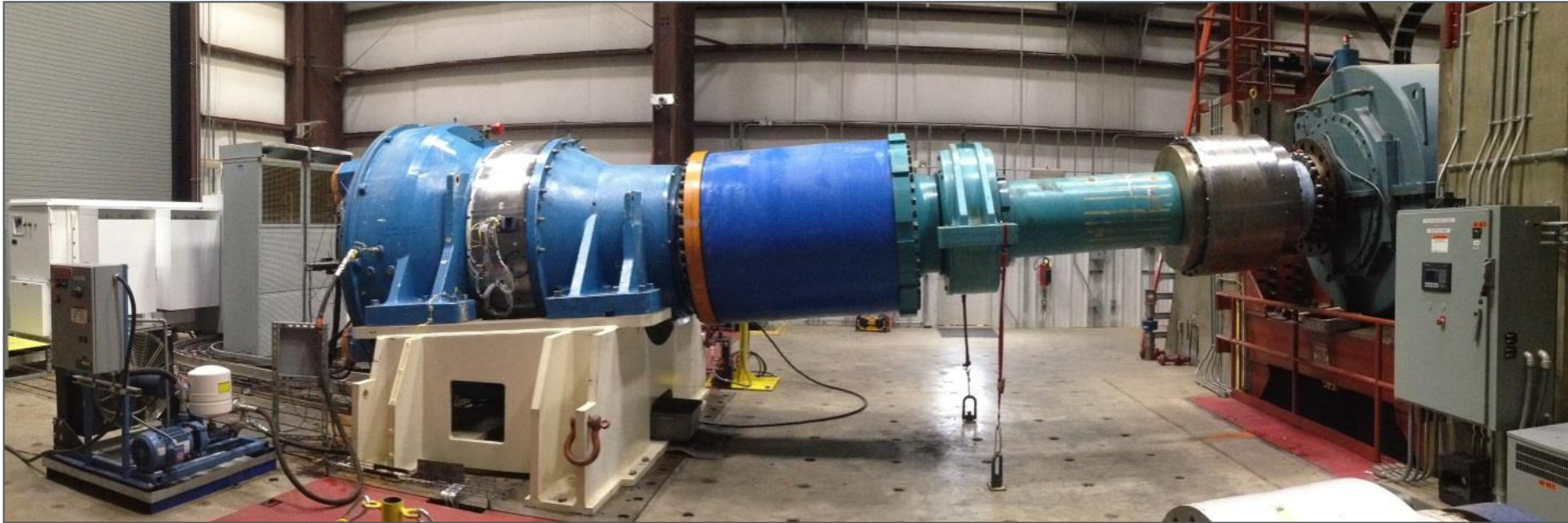
Next Generation Drivetrain in NWTC 2.5 MW Dynamometer
