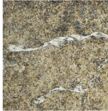
Roller with spall and white-etch crack
