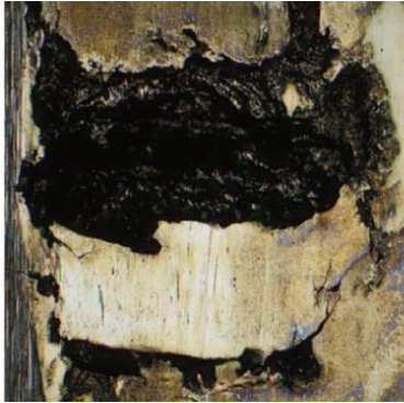
Roller with spall and white-etch crack
