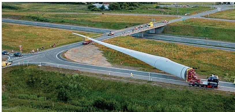
Figure 4b Transport of an 80-meter blade to a 7-MW test turbine in Scotland illustrates logistics challenges. 81
