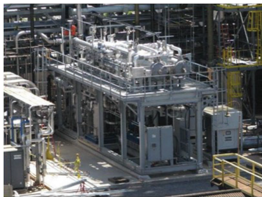
Figure 4.E.1 The 1 MW e , 20 ton per day MTR Membrane Module at the NCCC
