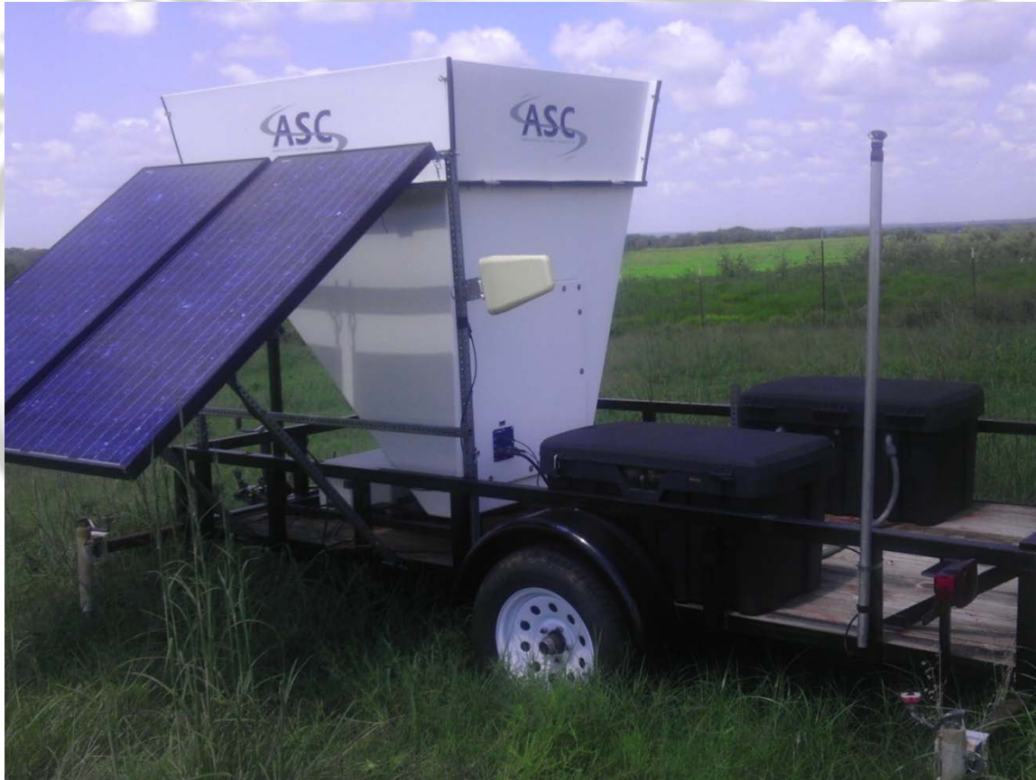
ASC SODAR Unit Solar Panels and Battery Packs
