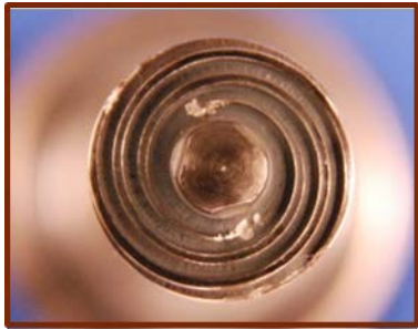
Pin with 3 Flats Double scrolled shoulder, Shoulder to pin ratio (S/P) =3
