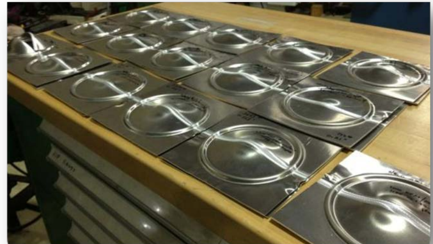
Pin with 3 Flats Single scrolled shoulder, Shoulder to pin ratio (S/P) =2.5
