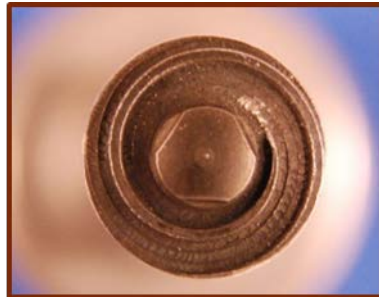
Pin with 3 Flats Single scrolled shoulder, Shoulder to pin ratio (S/P) =2.5
