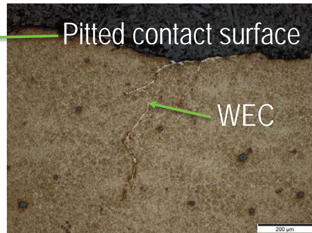
Etched circumferential cross-section
