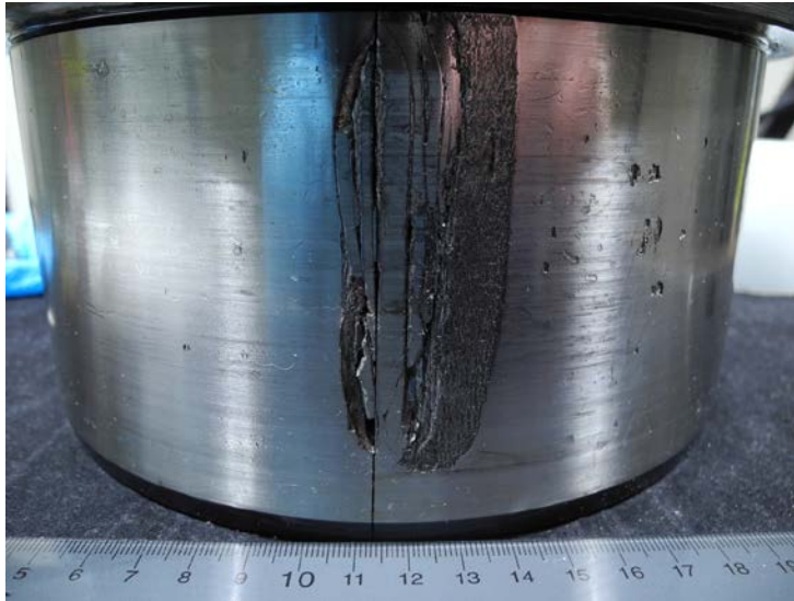
White-Etching Crack Bearing Failure
