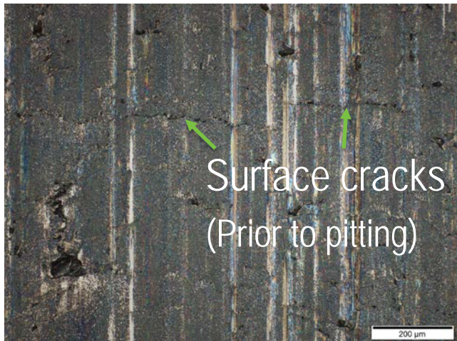
Examples of surface damage on test samples
