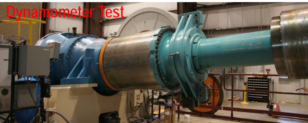
Dynamometer Test Develop new gearbox and power converter Reuse existing generator and main bearings
