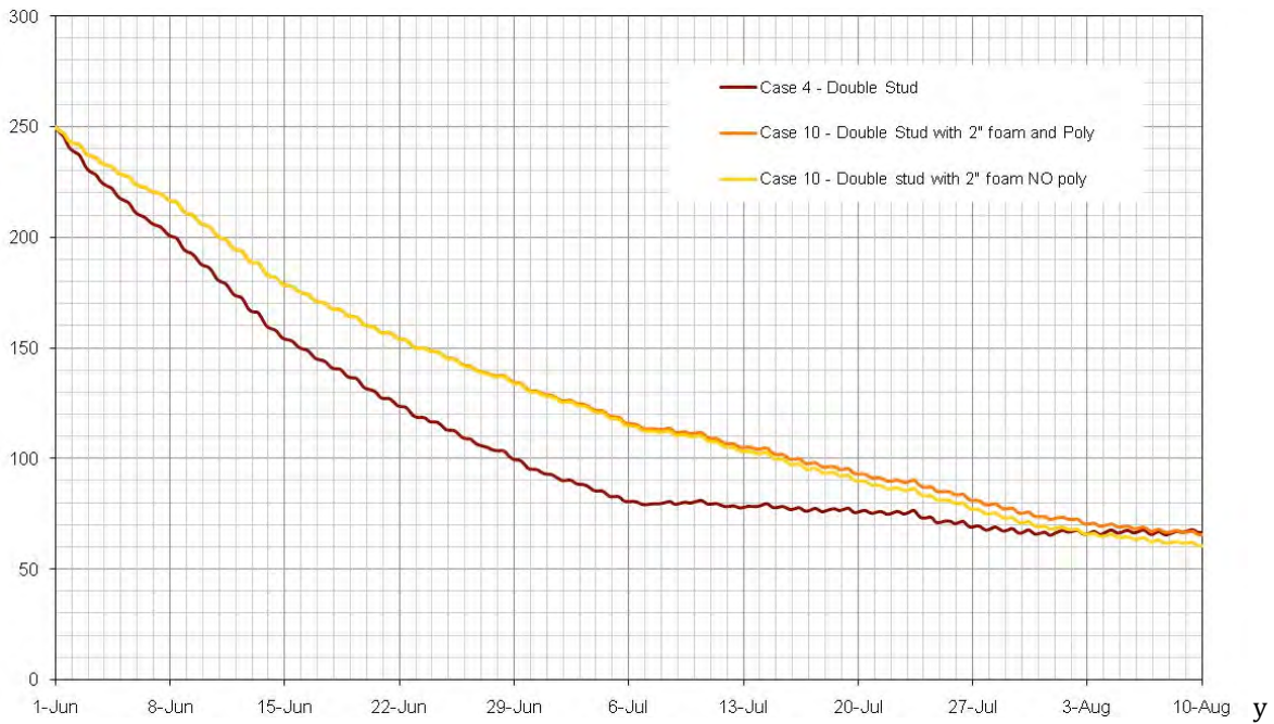
Figure 27 : Drying Curves for Case 4, and Case 10 with and without a poly vapor barrier
