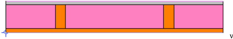
Figure 6 : Typical framing 16"o.c. - 9% framing factor
