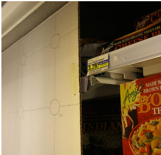
Figure 5. White test card inside of case with measurement locations
