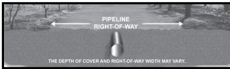
Figure 20: Typical Pipeline Right-of-Way Cross-Section ( https://www.aogc.com/beawarepipelinesinyourcommunity_en.aspx )
