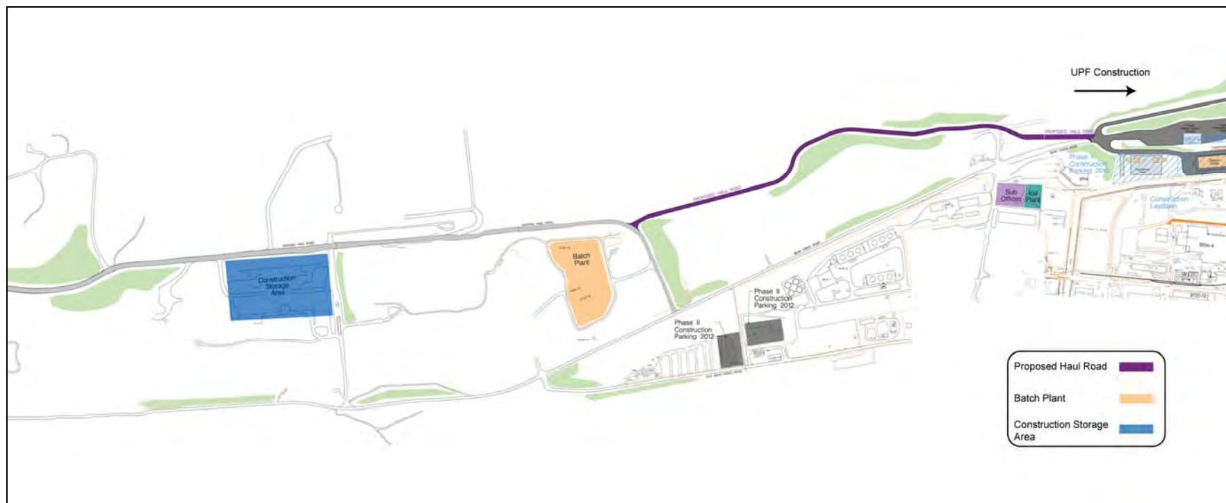
Figure 3.2.2-3. Temporary Haul Road, Batch Plant, Storage Area, and Temporary Parking for UPF Construction.
